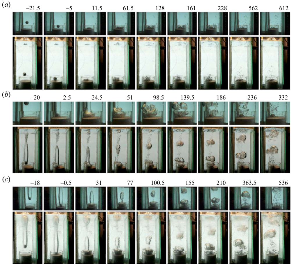
Figure 5. Impact dynamics of the projectile ( D_p = 40 mm) on the granular bed submerged in water for (a) E_k = 1.3 J ( \ell_B^{max} = 0 ), (b) E_k = 3.3 J (pinch-off of the air bubble in the bulk liquid; 0 < \ell_B^{max} < L_W ) and (c) E_k = 4.6 J (surface pinch-off at \partial A ; \ell_B^{max} \approx O(L_W) ). In each panel, the top image depicts the dynamics at the bed, and the bottom shows the dynamics over the entire liquid column captured using different cameras. The time, t in milliseconds (ms), is shown at the top of each panel, with t = 0 ms representing the instant when the projectile touches the granular bed surface.
