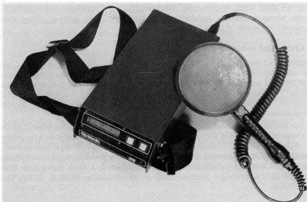
Figure 2 Circular head scanner and reading apparatus.
