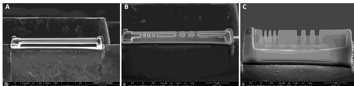
Figure 1. (A) Top-down view of sample after in-situ lift-out from Si, mounted and thinned, on the TEM half-grid. (B) Top-down and (C) Cross-sectional view of sample after fabrication.
