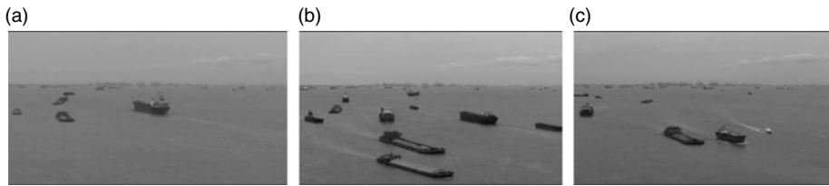
Figure 1. Typical frames of the collected image sequences for each ship detection scenario: (a) low traffic volume; (b) high traffic volume; (c) strong water clutter interference.
