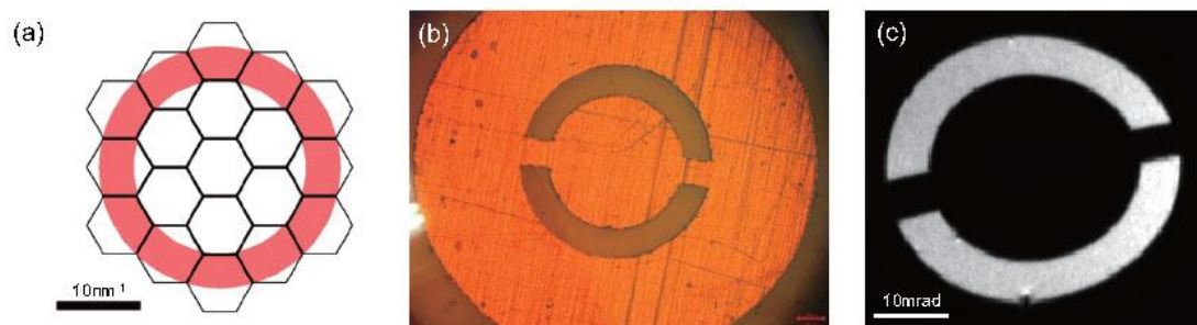
Figure 1. (a) An illustration of h-BN Brillouin zone and the collection area in reciprocal space. (b) The optical microscopy and (c) TEM image of annular aperture.
