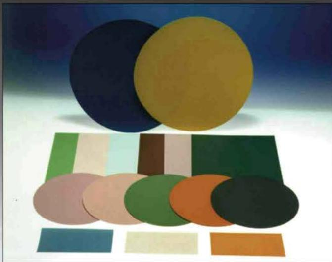
Lapping film consists of precision graded abrasive particles bonded to a flat, uniform polyester film backing. It provides excellent edge retention and maintains planarity across dissimilar materials.
