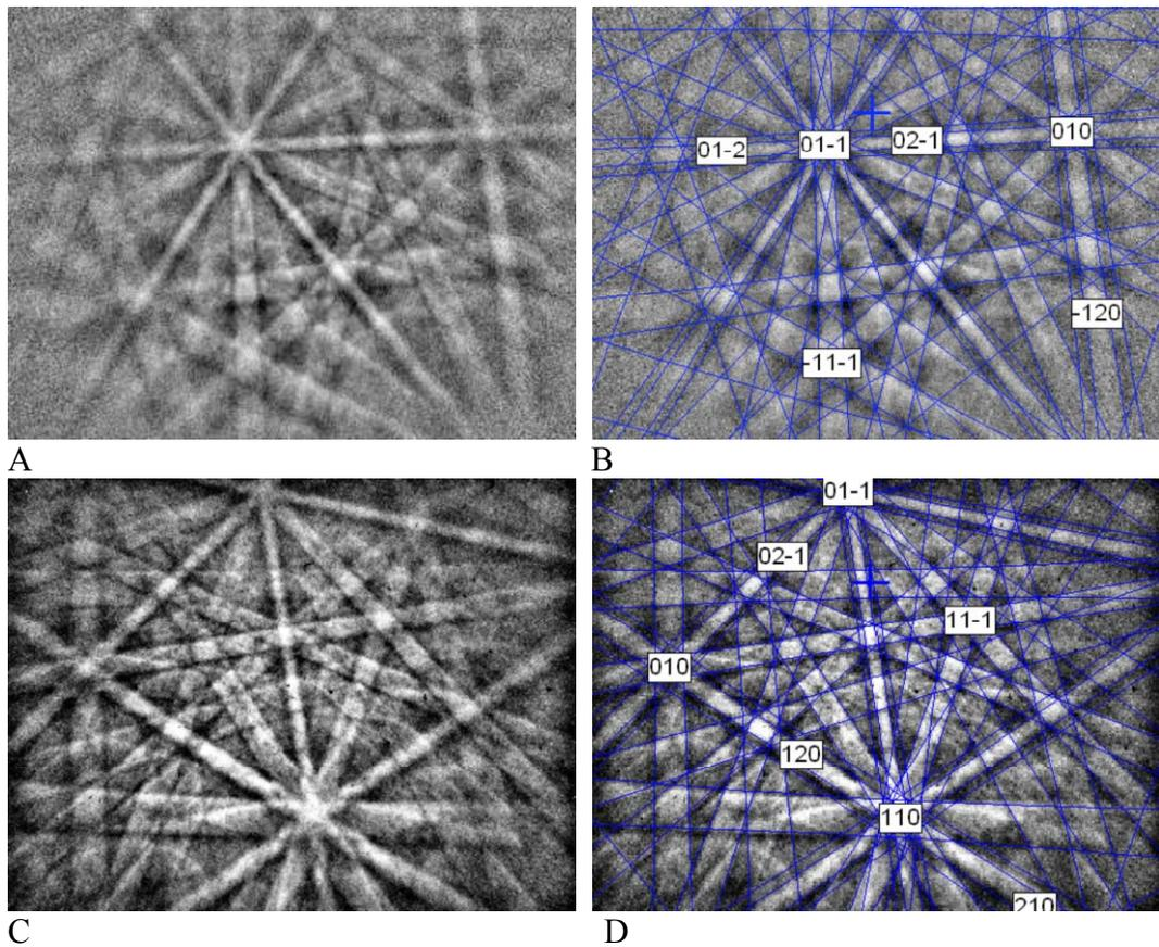
Figure 1. Indexed pattern of copper before (A & B) and after (C & D) ion polish. (B & D are indexed.)
