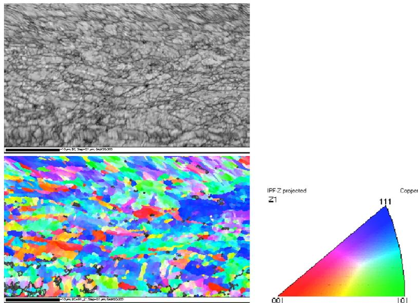
Figure 2. Band contrast image and Z-IPF colorization of copper cross-section in printed circuit board.
