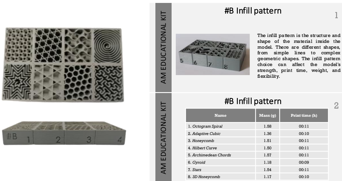
Figure 2. AM model for infill pattern
