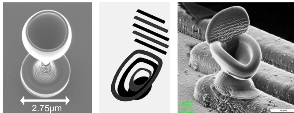
Fig. 1. Wine glass made by deposition (collaborative project with NEC & Univ. of Hyogo) (left), sliced 3D-CAD data (middle) and nano-toilet (right).
