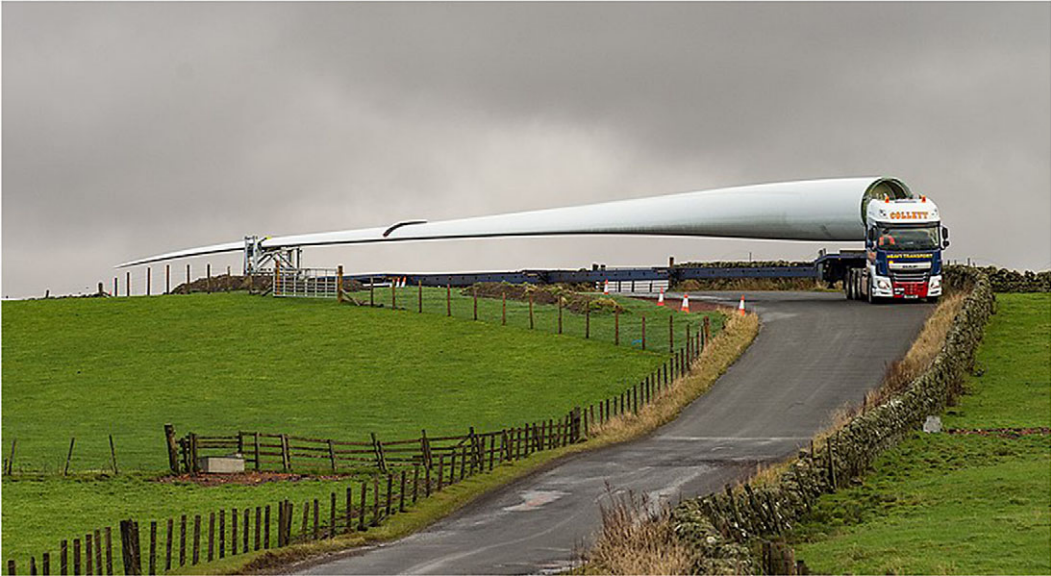
Figure 17. Transportation of blades (58.7 m long for GE 2.75–120 wind turbines) to Muirhall Onshore Wind Farm, South Lanarkshire (Photo credit: https://www.collett.co.uk/muirhall-wind-farm/ ).
