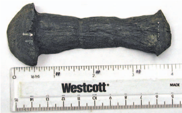
Figure 1: A macro photo of a hull rivet recovered from the wreck site. It shows a "woody" appearance due to the ferrite being corroded away, leaving ridges of slag. The right end head of the rivet has popped off, leaving a residue of the inside of the head.
