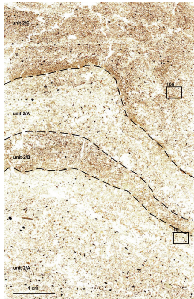
Fig. 6. High resolution scan of sample 2. Black boxes indicate location of micrographs depicted in Fig. 16e and l. Black dashed line indicates the boundary between discrete units.
