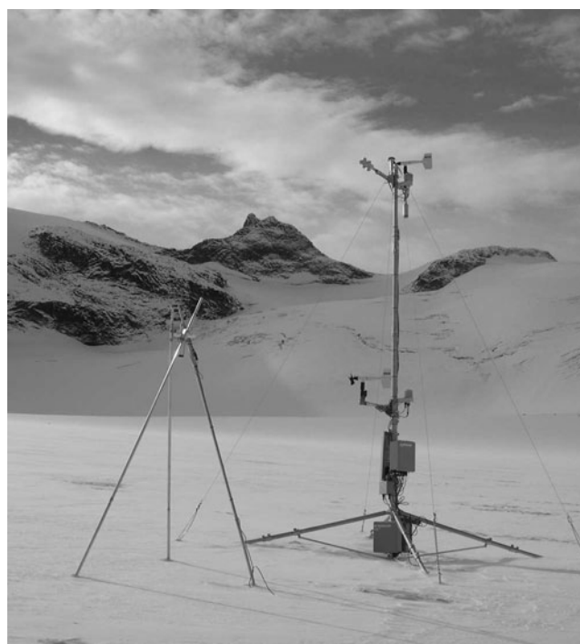
Fig. 2. The AWS at Storbreen. Measurements of relative humidity, temperature and wind are made at two levels above the ice surface. The tripod to the left measures surface height.
