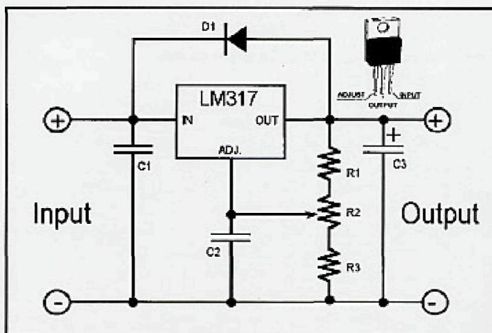
Circuit diagram for stable voltage source to replace mercury batteries
