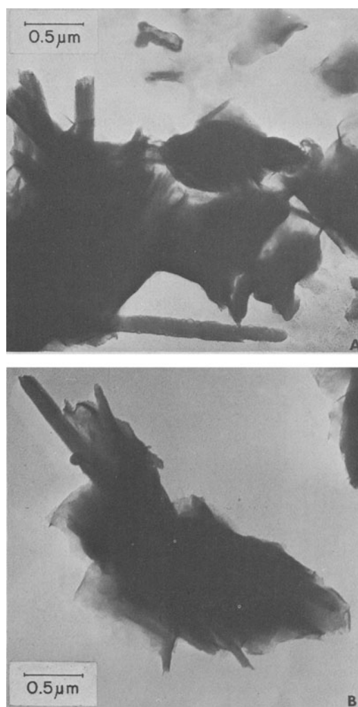
Fig. 5(a) and (b). Aggregations of lath-shaped units with montmorillonite in a bentonite from North Africa.
