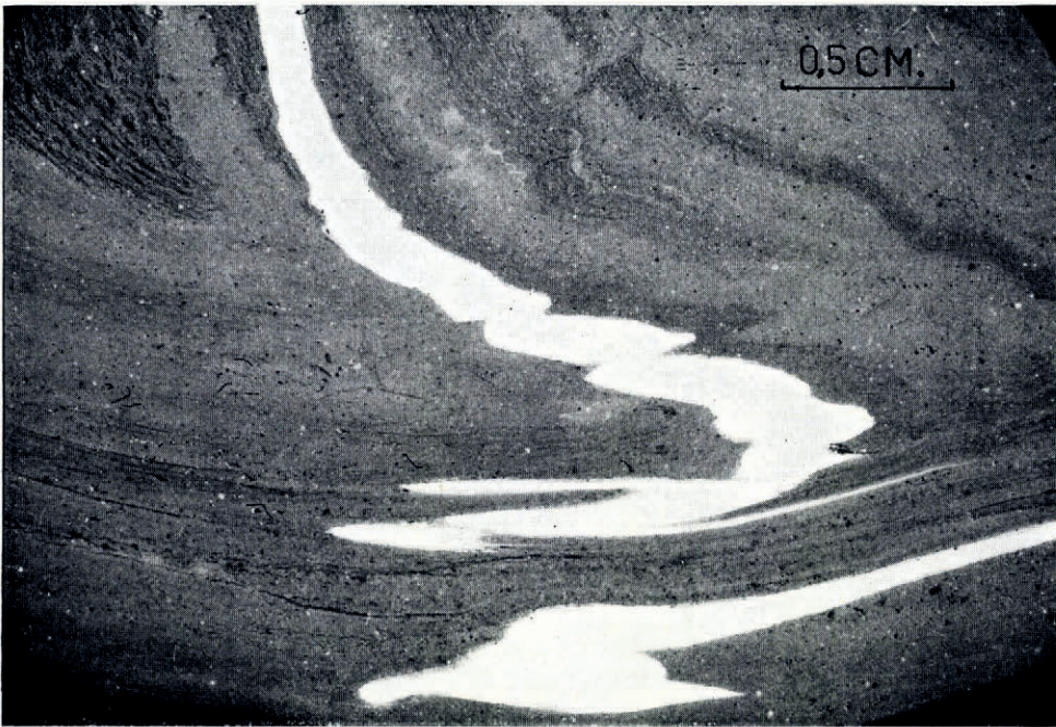
Fig. 9. Detail of part of a centrifuged piedmont-glacier model of heterogeneous bouncing putty. Compare this structure with the Malaspina Glacier structure in Figure 11
