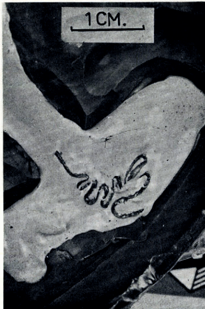
Fig. 8. Layer of competent stitching wax buckled in a centrifuged model of a piedmont glacier of bouncing putty. The stitching wax is considerably more viscous and stiff than any of the enclosed layers in the other models. Note in this connection the smooth rounded outline of the folds
