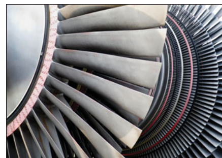
Turbines for power generation have complex, precise geometries, and are manufactured using difficult-to-machine high-temperature alloys.
