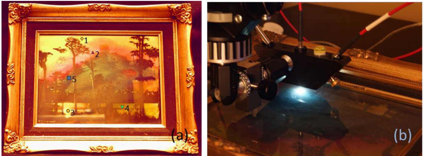
Figure 1. (a) Orotone photograph attributed to E. G. Barnhill, (b) Microfadeometric analysis in progress
