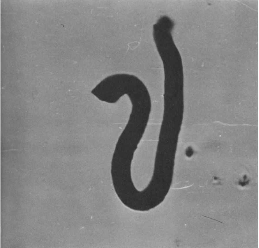
FIGURE 5.—An optical micrograph of a kaolinite “stack” over 100 microns in length. Although the resolution in this view is not sufficient to show the details, this piece is made up of hundreds of layers arranged as is shown in Figure 4.
