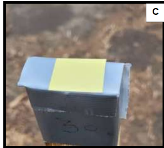
Figure 2. (A) Back-and-forth operating procedure in which deposition of the left-wing overlaps with that sprayed by the right-wing. (B) Water sensitive papers positioning in the open field and on the (C) wooden block
