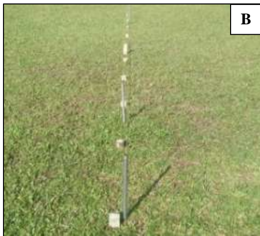
Figure 2. (A) Back-and-forth operating procedure in which deposition of the left-wing overlaps with that sprayed by the right-wing. (B) Water sensitive papers positioning in the open field and on the (C) wooden block
