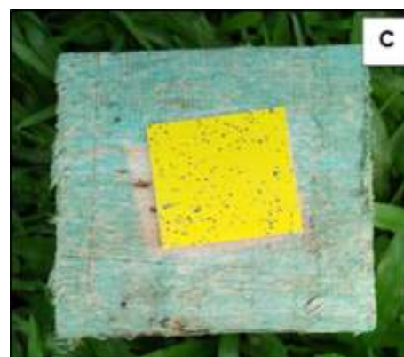
Figure 4. Droplet analysis using (A) Snap Card application and (B) ImageJ software and (C) Spraying deposition on WSP paper
