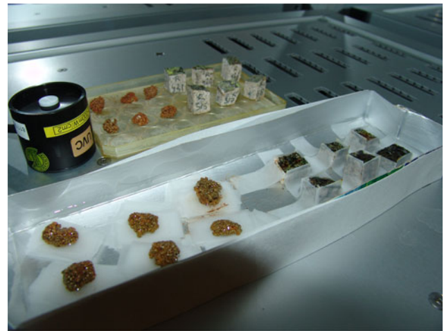
Fig. 3. Irradiation chamber with the samples in the center of the irradiation area and the sensor located close to them. In the left front thalli of C. gyrosa are located on water soaked paper pads, in the right front there are cutted stones with crustose thalli of R. geographicum wetted by adjacent paper strips. The dry samples are depicted on a plastic tray in the center with six samples each of C. gyrosa (center left) and R. geographicum (center right).
