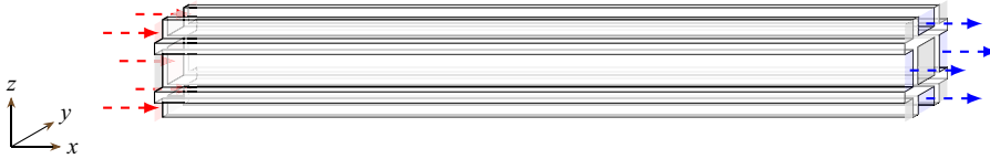
Figure 1. The four-channel set-up of one central inflow (red) channel with fractions of surrounding inflow (red) and outflow (blue) channels separated by porous walls. Grey, no-slip walls. The sketch is scaled for improved visual clarity.
