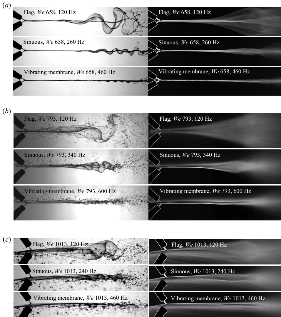
Figure 6. Lateral views of the sheet showing three wave profiles leading to flapping flag, sinuous and vibrating membrane instability, for (a) 2\theta = 60^\circ , (b) 2\theta = 90^\circ and (c) 2\theta = 120^\circ . The vibrating membrane is a special case of sinuous instability in which the sheet is unaffected but a large section of the sheet surface shows very small-amplitude perturbations, similar to the vibrating thin membrane. The SPL level in all cases is 110 dB. See also supplementary movie 1, available at https://doi.org/10.1017/jfm.2021.251 .
