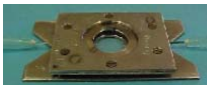
FIG. 1a. Metal flow chamber used to grow biofilms under flow conditions.
