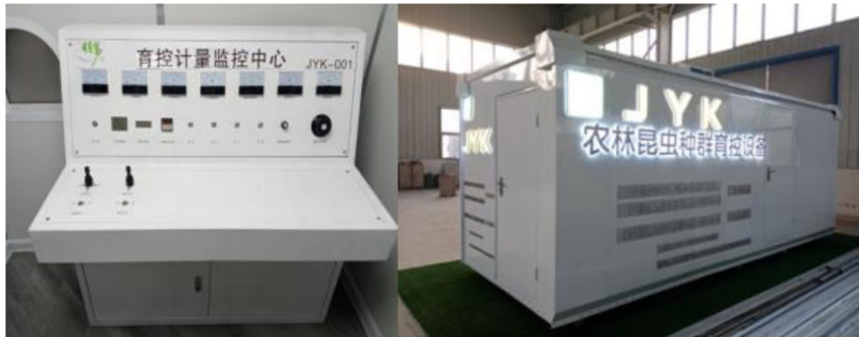
Figure 1. The X-ray irradiator used in this study. The irradiator (JYK-001 type) was independently developed by Hebi Jiaduoke Industry and Trade Co., Ltd, Hebi, China. (Left) Outside view of the X-ray irradiator and (Right) the platform for the manipulation of irradiation.
