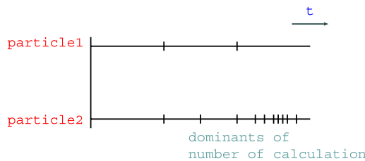
Figure 3. If we adopt the individual timestep method, the small steps part dominates the calculation.
