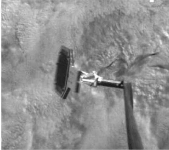
Figure 23. Target snapping off the end of the boom.
