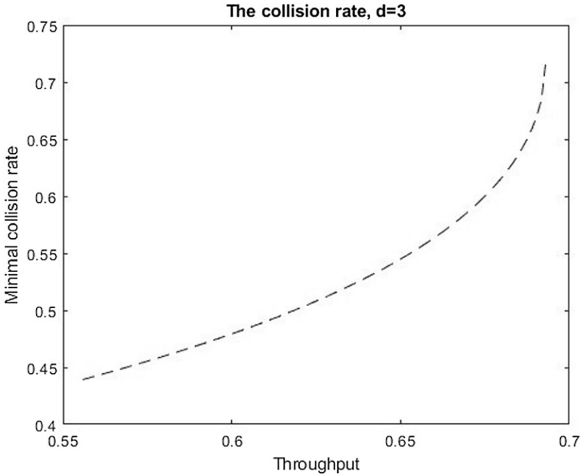
FIGURE 2. The minimal obtainable collision rate, constrained by achieving a certain throughput rate. The figure was obtained numerically using a standard solver for constraint non-linear optimization problems. p^{bi} was used as the initial value.
