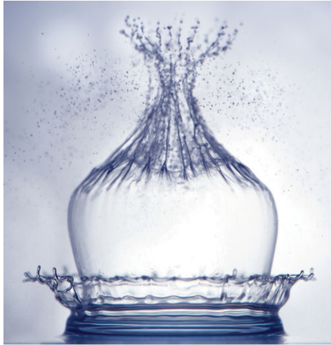
Figure 1. Example of the double crown, for a glycerine drop of diameter D = 4.47 mm, impacting at U = 7.75 m s -1 onto a 0.8 mm thin layer of silicone oil of viscosity 2 cSt. This corresponds to dimensionless parameters: Re_d = 36 , Re_f = 17\,420 , We_d = 5285 , We_f = 13\,125 and \delta/D = 0.18 . This snapshot of the ephemeral form is shown 3.18 ms after first contact of drop with pool surface. The drop contains dye causing the blue hue at the base of the crown.
