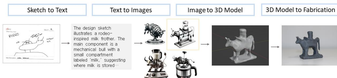
Figure 1. Our Sketch2Prototype framework which takes in a conceptual design sketch as input, and produces multiple inspired images, a 3D model, and finally a fabricated prototype
