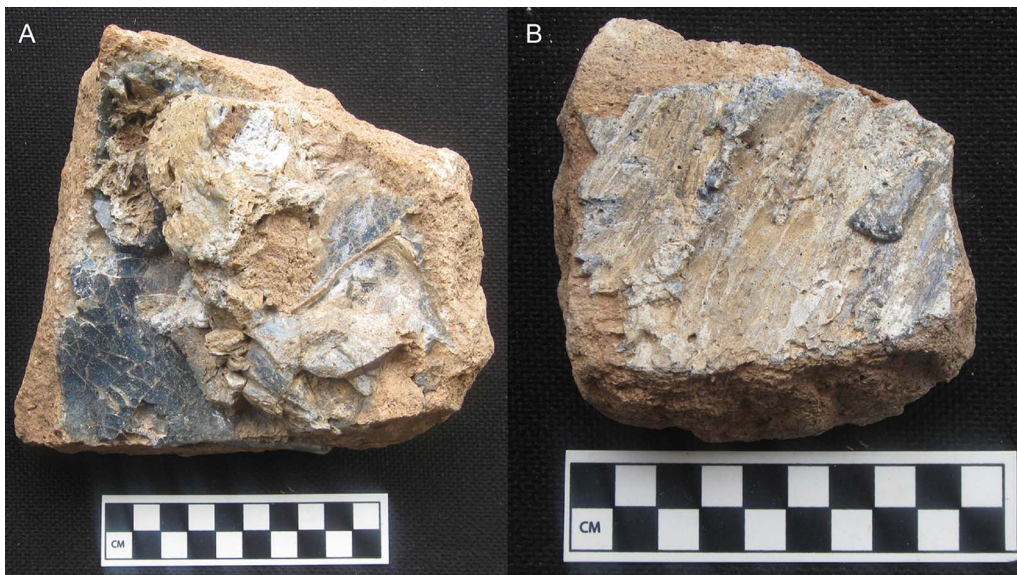
Figure 2. Crucible fragments from Natural History Museum storage with suspected semi-finished glass: A) (sample IF0108) the well-made glass layer beneath the chunk of the semi-finished glass indicates that the crucible must have been used multiple times in glass production; B) (sample IF0113) the striations in the glass surface indicate scraping out of the soft glass paste while it was still hot, a common observation on many crucible fragments from Ile-Ife (figure by Abidemi Babalola).
