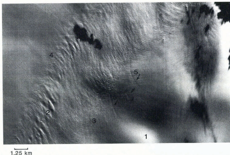
Fig. 4. Up-glacial end of the snake. Mottles (1) occur on the righthand side of the image. A train of lumps (2) is located on the lefthand side. Hook-shaped en échelon trains of crevasses run from top center to lower left on either side of the snake (3 and 4). Two long curved crevasses of unclear origin occur in the middle of the figure (5). Dark spots are cloud shadows. Flow is toward the bottom of the figure. Scene width is 20.00 km.
