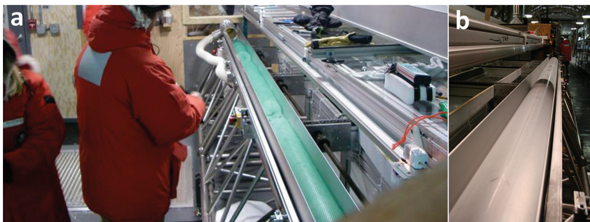
Fig. 11. View of the 'Receiving and logging' station at WAIS Divide with (a) 2.5 m of brittle ice contained in the green elastic netting and (b) a 3.2 m long continuous run of ductile ice showing one of the many prominent tephra layers observed in the WAIS Divide ice core.
