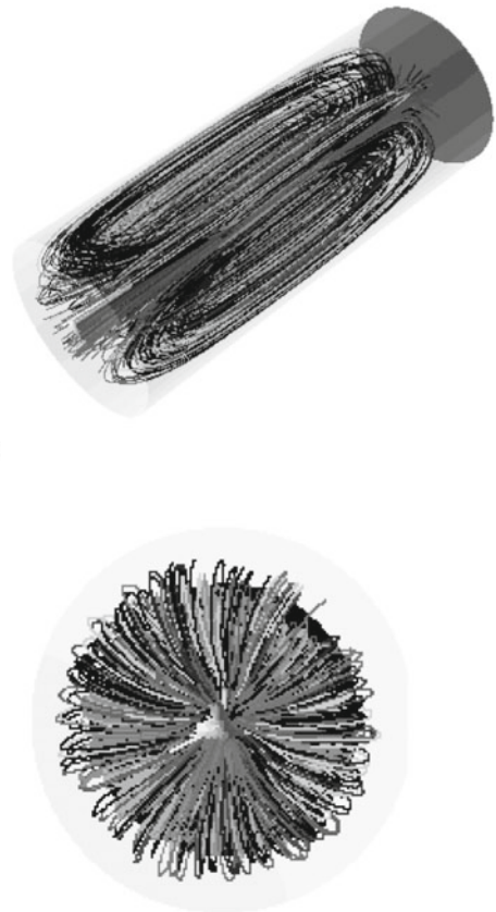
Fig. 4. Runs of streamlines in the reactor. Methane oxidation was not considered.
