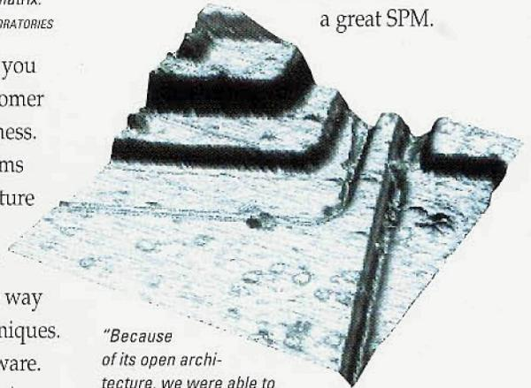
*"Because of its open architecture, we were able to integrate our Explorer SPM into our test system for contactless electrical characterization of integrated circuits. We conduct function and failure analysis of analog and digital devices with both high-spatial and temporal resolution. This is a 20µm topography image of a part of an integrated transistor with gate and gate contact."*
