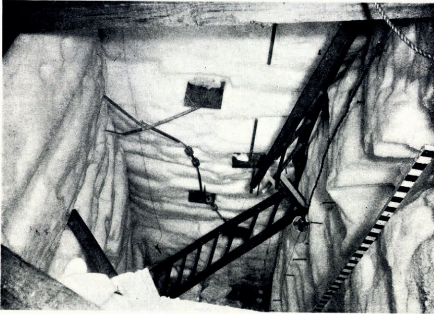
Fig. 2. Glaciological pit at Little America III, dug in 1940 by Wade. The ladder broke because of contraction to pit due to settling of firn. Compression meters in north wall L_1 (top right), L_3 (below, partially hidden by ladder), L_2 (displaced to the left). Vertical row of nails, placed by Howard in 1947 in east wall (right part of photo). Compare with plate I in Howard's report (1948). Photograph 17 November 1957 by H. C. Hoinkes
