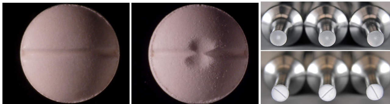
Figure 1. Left panel: normal tablet; Middle panel: tablet with depression; Right panel: Upper punch faces (top) and lower (bottom) punch faces after 500 cycles that have adhered tablet material.
