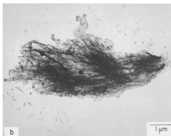
Figure 4. Typical smectite aggregates formed during the hydrothermal treatments at 316°C and 1379 bars (a) in the system sepiolite/CaCl 2 , and (b) in the system sepiolite/NaCl.
