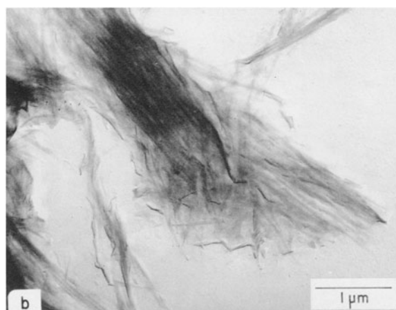
Figure 3. Typical smectite particles formed during the hydrothermal treatment at 260°C and 69 bars (a) in the system sepiolite/CaCl 2 and (b) in the system sepiolite/NaCl.
