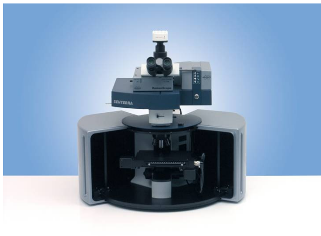
Figure 1. Senterra Raman Microscope.
