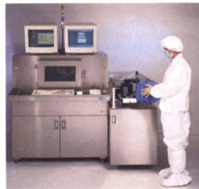
Dimension 9000 AFM: The first fully automated AFM for semiconductor metrology.
