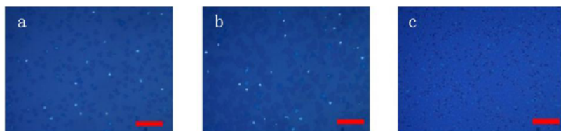
Figure 5. Optical images of WSe 2 with different growth pressures: (a) 280 Pa, (b) 180 Pa and (c) 70 Pa. All the scale bars are 20 μm and the temperature used for the pressure dependency study is 765°C.
