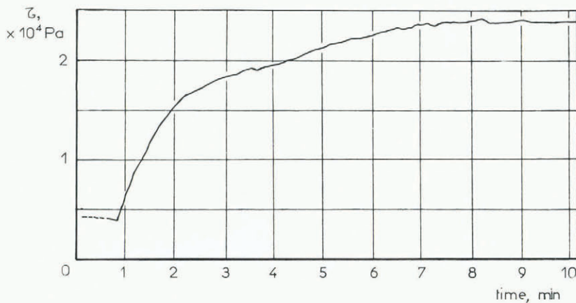
Fig. 10. Mechanical bevametre, relation between shear stress and time for snow B, with normal stress of 8.5 \times 10^2 Pa, and rotation rate r_r = 0.0075 r.p.m. ( 1.25 \times 10^{-4} Hz). The first part of this test, which is not represented here, was carried out at 0.0075 r.p.m. with no failure, followed by a relaxation.
