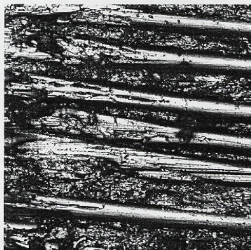
Figure 2 Wear surface of a glass fiber reinforced polymer composite material (120 x 120 \mu\text{m} ). Supplied by A Goninan & Co. Ltd.
