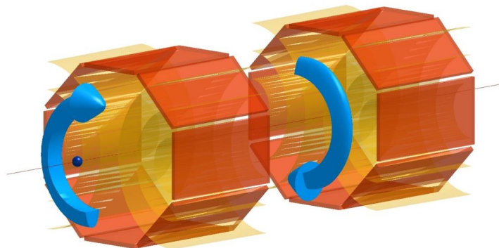
Fig. 2 A new cluster size filtering system introducing two rotating electric fields reversing each phase.
