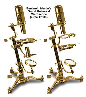
rack and pinion gears for the mirror and stage. The eyepiece is composed of two plano-convex lenses that are adjustable with another rack and pinion gear set. The most complex part of the Grand Universal microscope is the elaborate stage, which is really two stages connected together by means of a "U"-shaped bar. See: micro.magnet.fsu.edu/primer/museum/granduni.html
