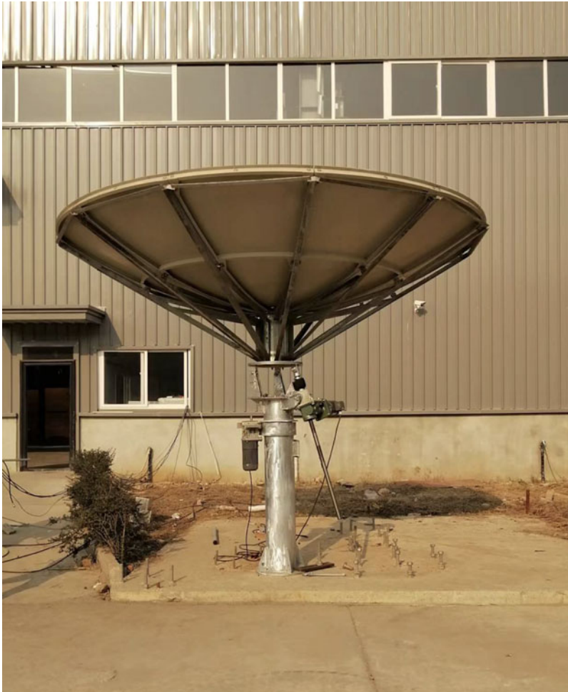
Figure 3. Photo of the Nigeria 3.7m radio telescope at the manufacturer's site undergoing drive tests.
