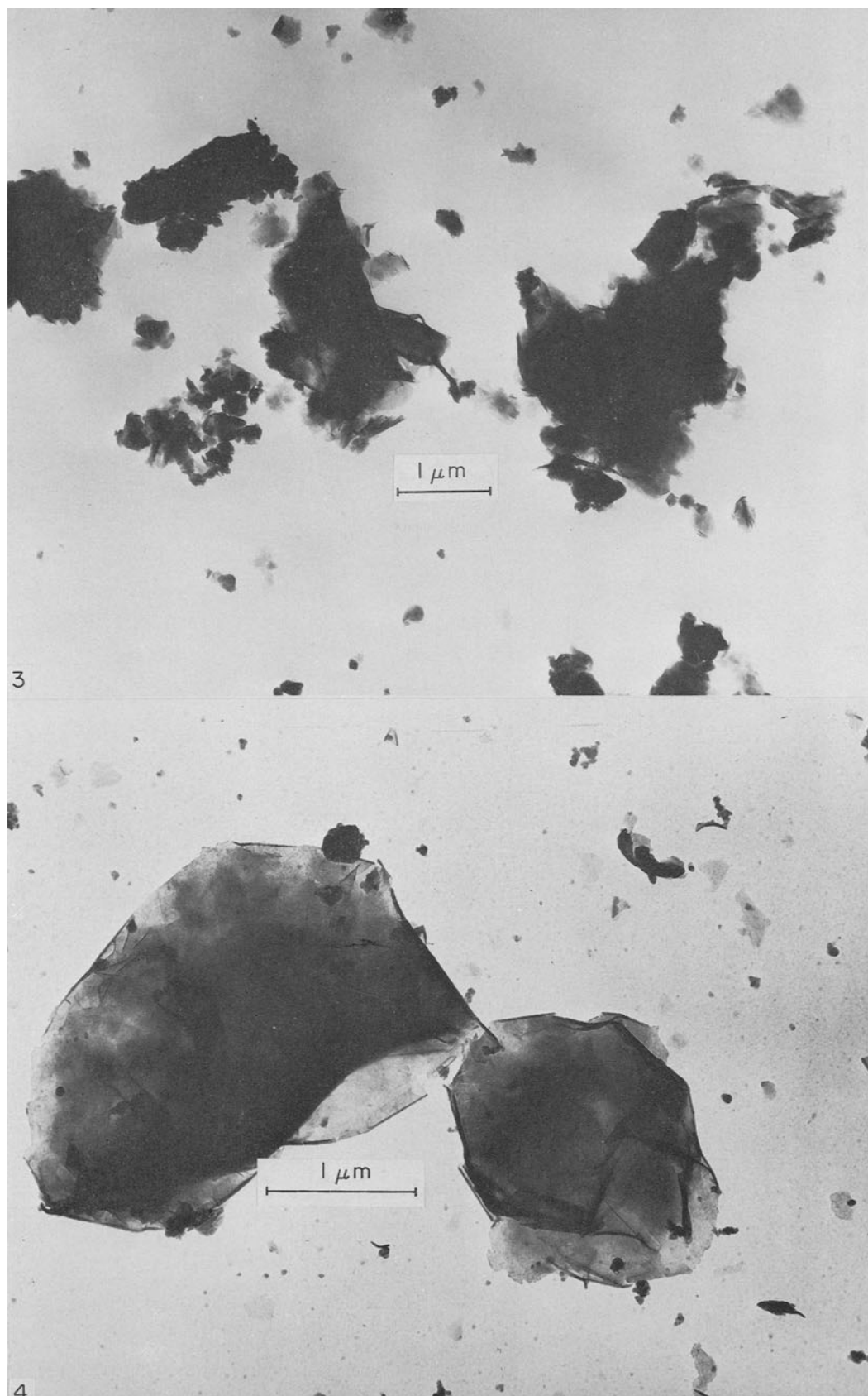
Fig. 3. Electron photomicrograph of dibenzylammonium montmorillonite (100 per cent exchanged). Magnification 24,000 \times .
