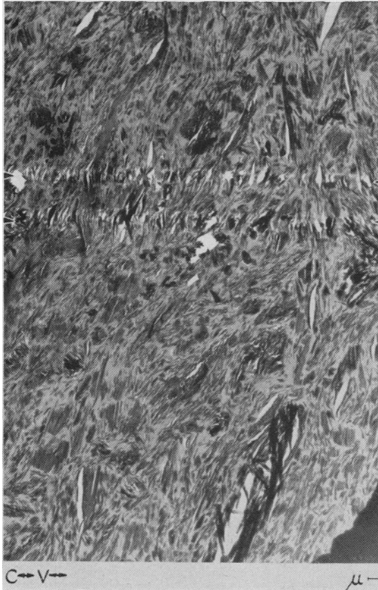
PLATE 4. Consolidated kaolin, a vertical section cut vertically.
