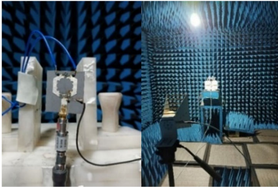
Figure 15. Measurement setup of the proposed RFA antenna.
