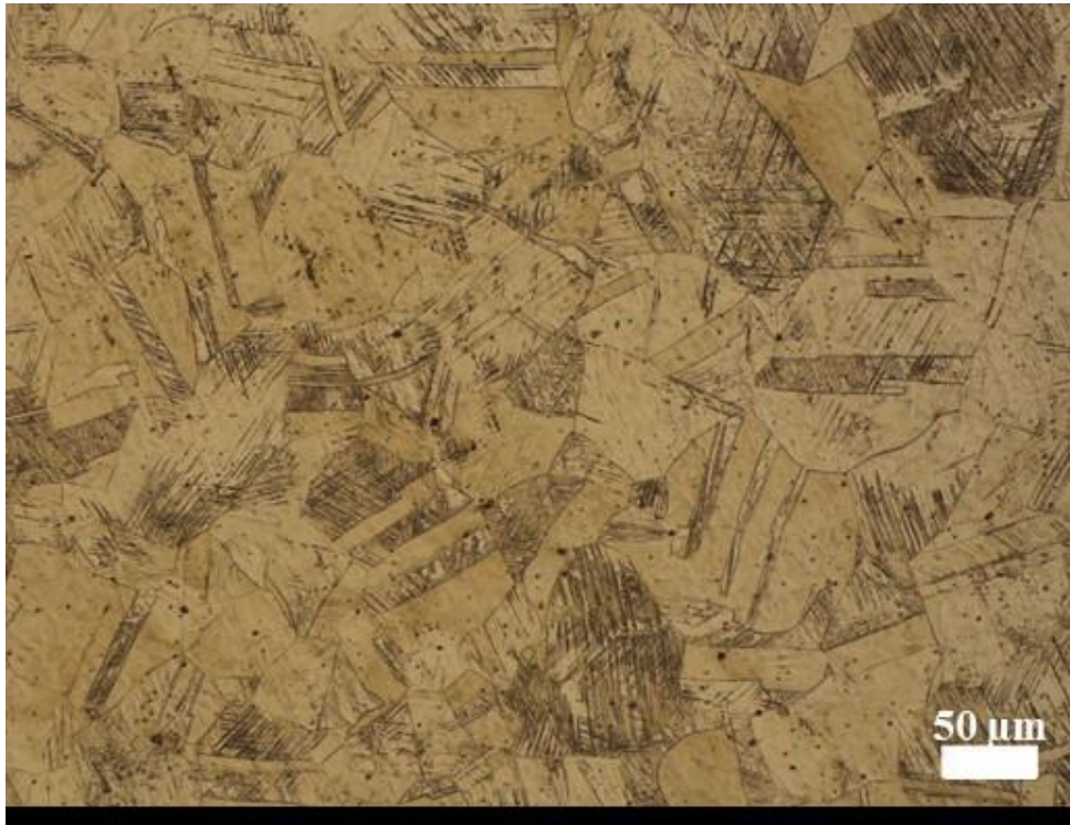
Figure 1. Bright field of optical micrographs at 200x magnification in the AISI 304 stainless steel using “aqua regia” ( \text{HNO}_3+\text{HCl} ) as the chemical etching.
